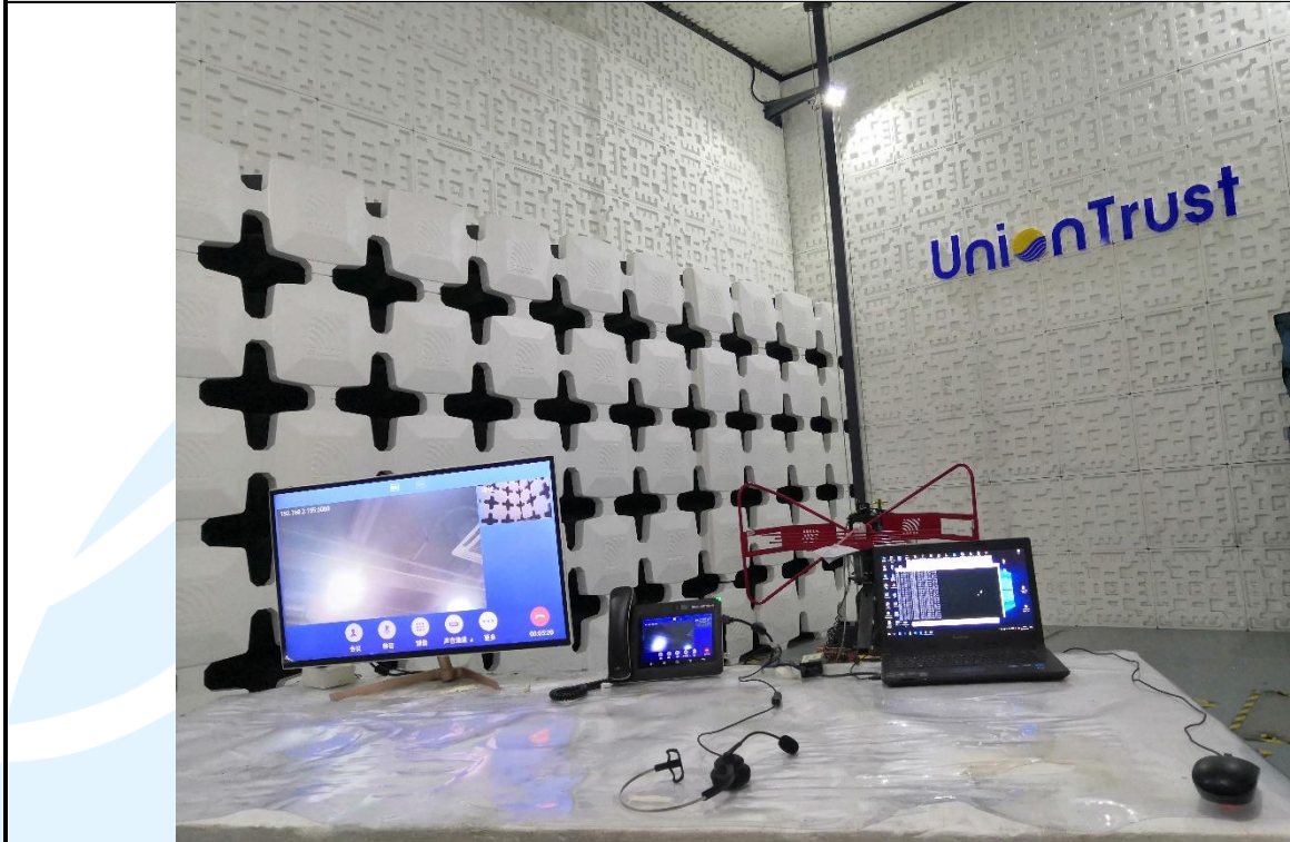
Radiated emission Test Setup (30 MHz~1 GHz)
