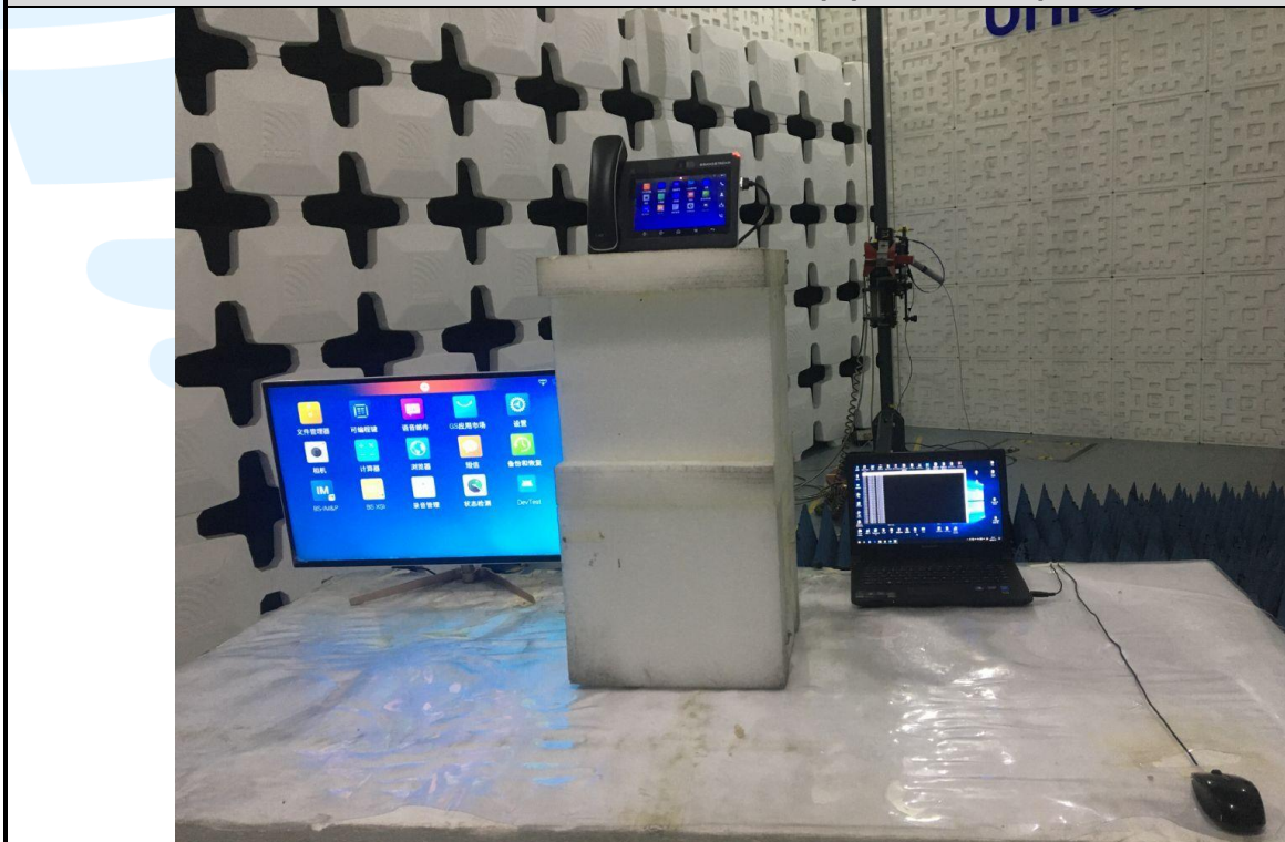
Radiated emission Test Setup (Above 1 GHz)
