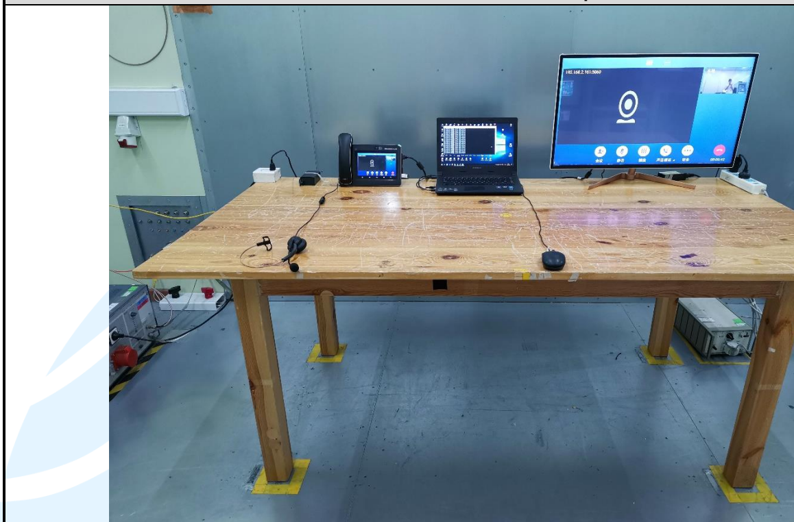
Conducted Emission Test Setup
