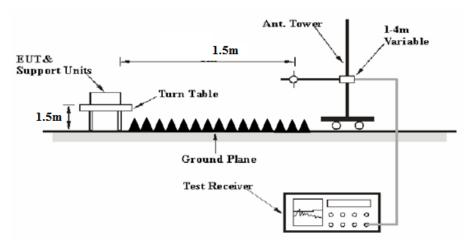
The radiated emission tests were performed in the 3 meters chamber test site, using the setup accordance with the ANSI C63.10-2013. The specification used was FCC 15.209, FCC 15.407 limits.
