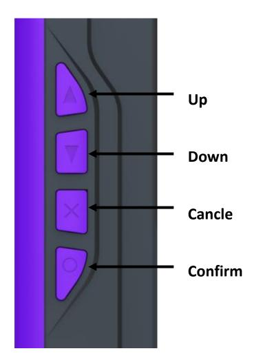
Flip up: arrow key, press this key to flip up the displayed menu. Scroll down: arrow key, press this key to scroll down the displayed menu. Cancel: Press the cancel button to cancel or return to the previous menu. Confirm: Confirm button to confirm the current operation.
