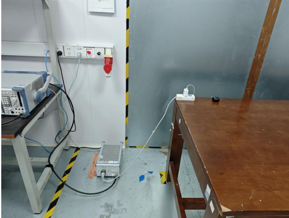
Conducted emissions at AC power line (150kHz-30MHz)
