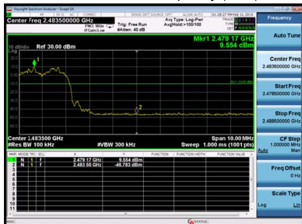
BT 3DH5 CH78, Carrier frequency (MHz): 2480
