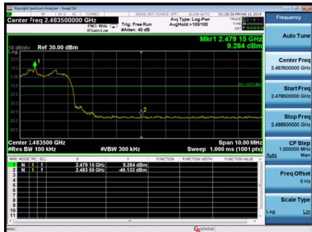
BT 3DH5 CH78, Carrier frequency (MHz): 2480
