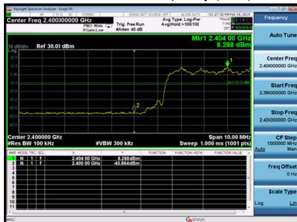
BT 3DH5 CH0, Carrier frequency (MHz): 2402
