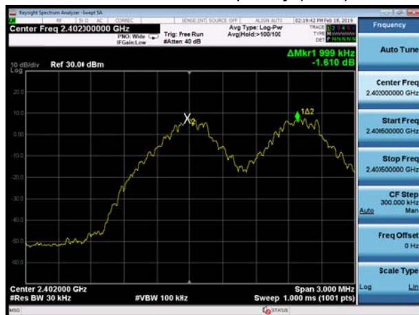
BT DH5 CH39, Carrier frequency (MHz): 2441
