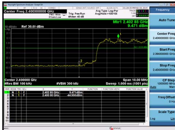
BT 3DH5 CH0, Carrier frequency (MHz): 2402
