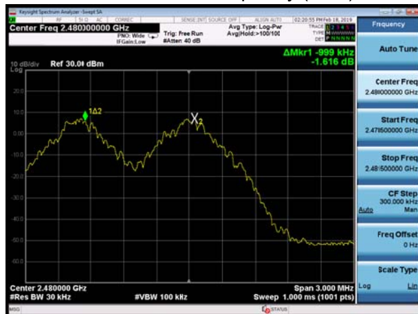
BT DH5 CH78, Carrier frequency (MHz): 2480
