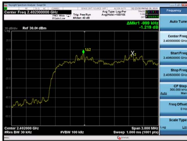
BT 3DH5 CH78, Carrier frequency (MHz): 2480
