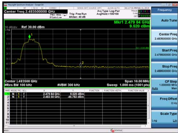
BT 3DH5 CH78, Carrier frequency (MHz): 2480
