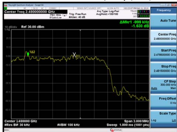
BT 2DH5 CH78, Carrier frequency (MHz): 2480
