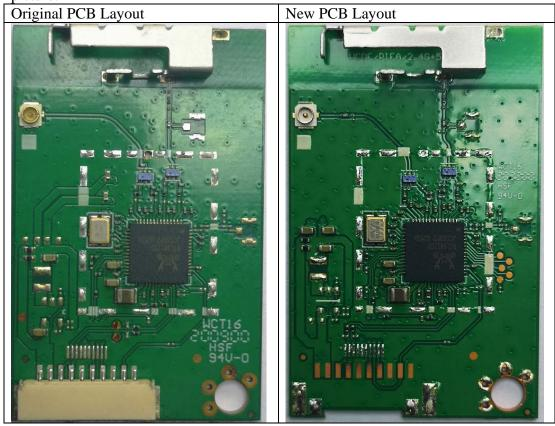
2. Added the new model WC16R2601, these model are electrically identical and only differ in model name and power supply port. Please refer to below picture:
