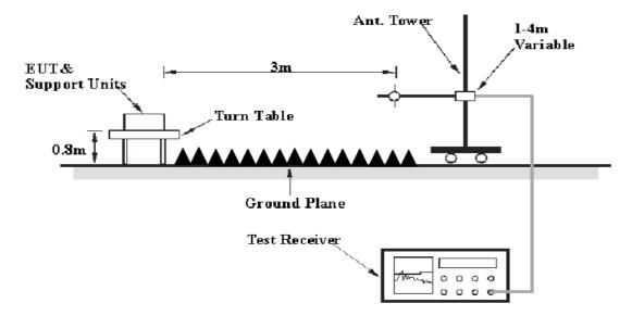
The radiated emission tests were performed in the 3 meters chamber test site, using the setup accordance with the ANSI C63.4-2014. The specification used was the FCC Part 15.109 Class B limits.
