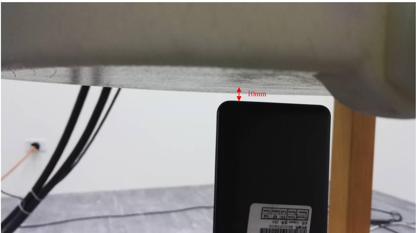
Body-worn Bottom Setup Photo (10mm)
