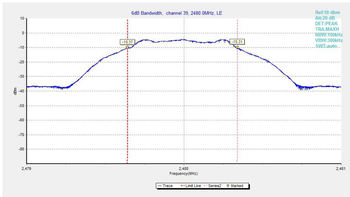
Fig.22. 6dB Bandwidth: GFSK, 2480 MHz
