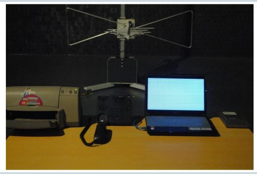
Radiated Emission test view (Frequency above 1GHz)
