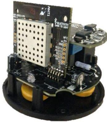
The DCC127 series photocontrol will use this DTL01 bluetooth board in order to communicate to the keyfob DTL02.
