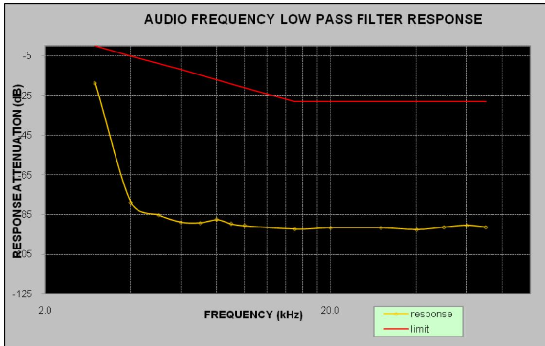
**FCC §2.1049 & §22.357 & § 22.731 & §74.462 & § 80.205 & § 80.207 & §80.211 & §90.209 & §90.210 – OCCUPIED BANDWIDTH & EMISSION MASK****Applicable Standard**
