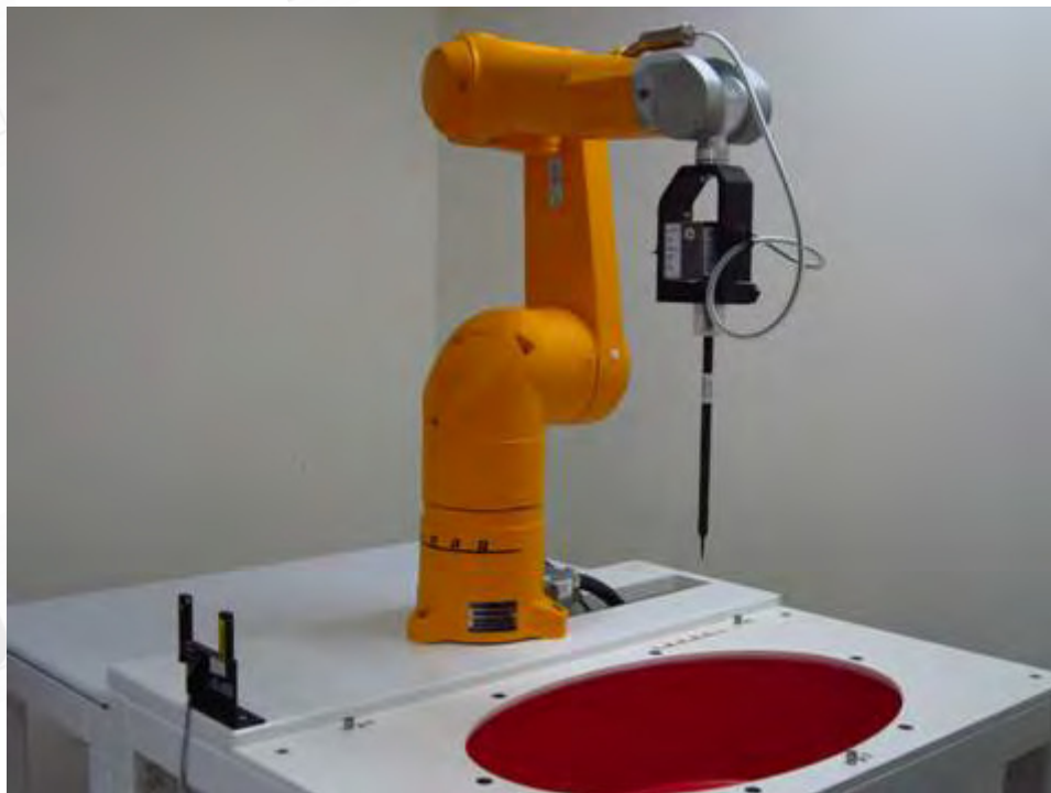
Fig.1 Photograph of the SAR measurement system
