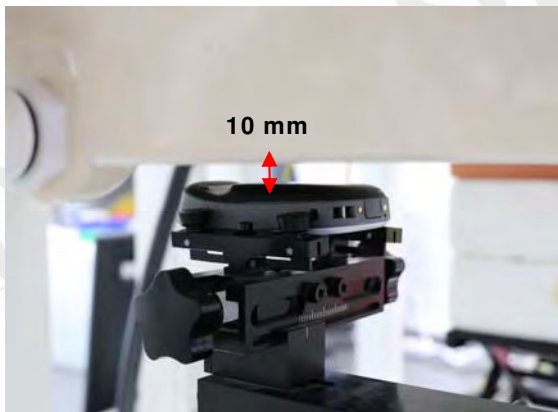
Fig.4 EUT Back side to flat phantom
