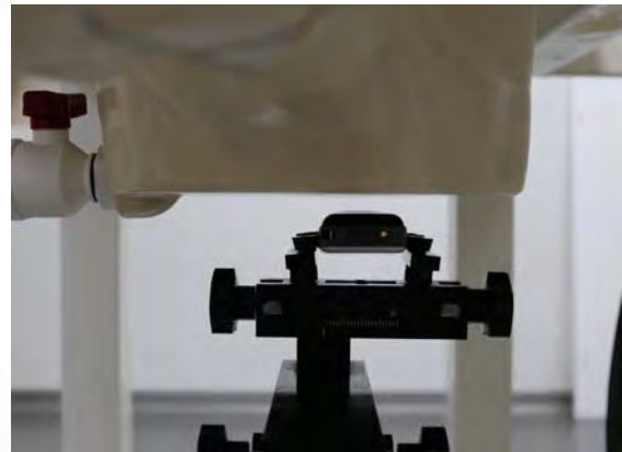
Fig.4 EUT Back side to flat phantom
