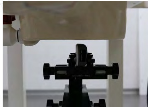
Fig.6 EUT Left side to flat phantom
