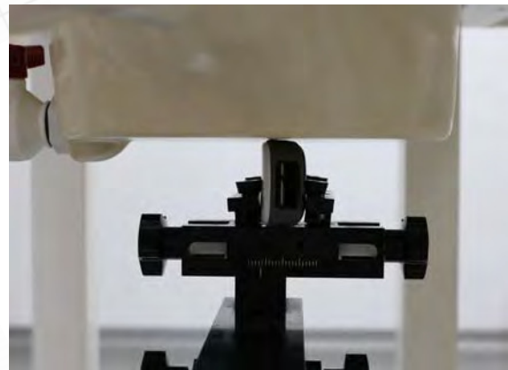
Fig11 EUT Left side to flat phantom
