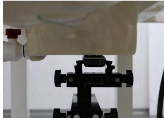
Fig.8 EUT Front side mode to flat phantom
