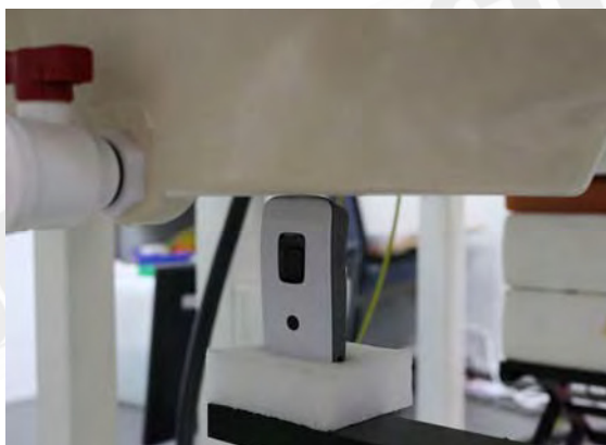
Fig.10 EUT Top side to flat phantom
