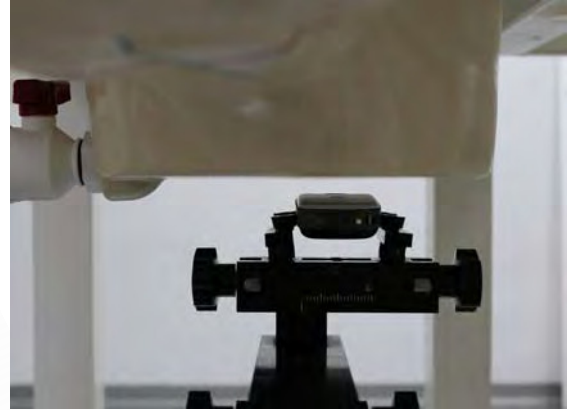
Fig.3 EUT Front side to flat phantom
