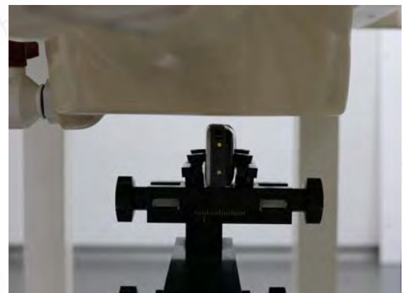
Fig.7 EUT Right side to flat phantom
