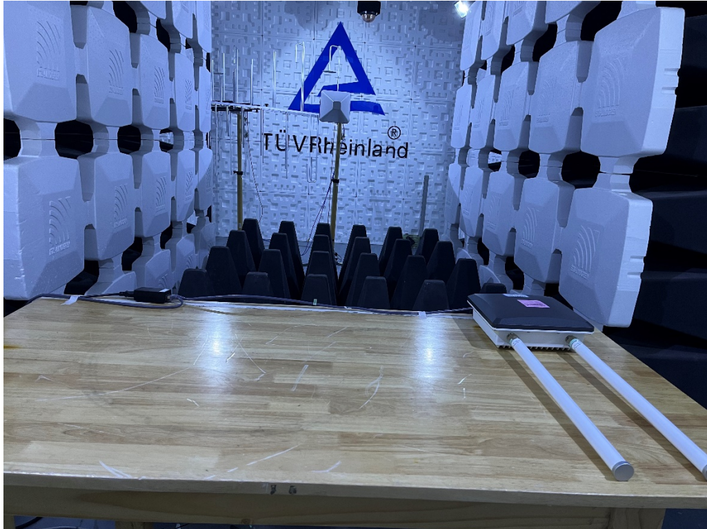
Photograph 3: Set-up for Radiated Emissions, above 1GHz
