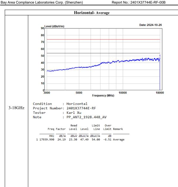
Note: Spectrum Analyzer Setting: RBW=1MHz, VBW=5kHz
