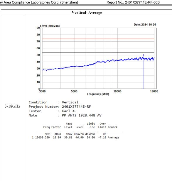
Note: Spectrum Analyzer Setting: RBW=1MHz, VBW=5kHz
