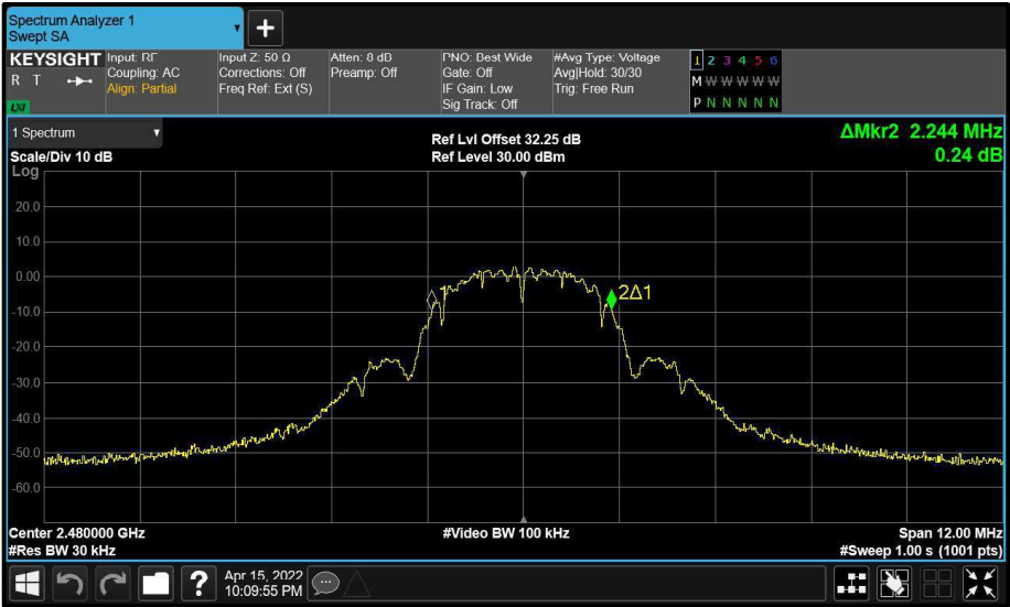
Figure 11 - A (A) 2480 MHz (CH26) 99% Bandwidth
