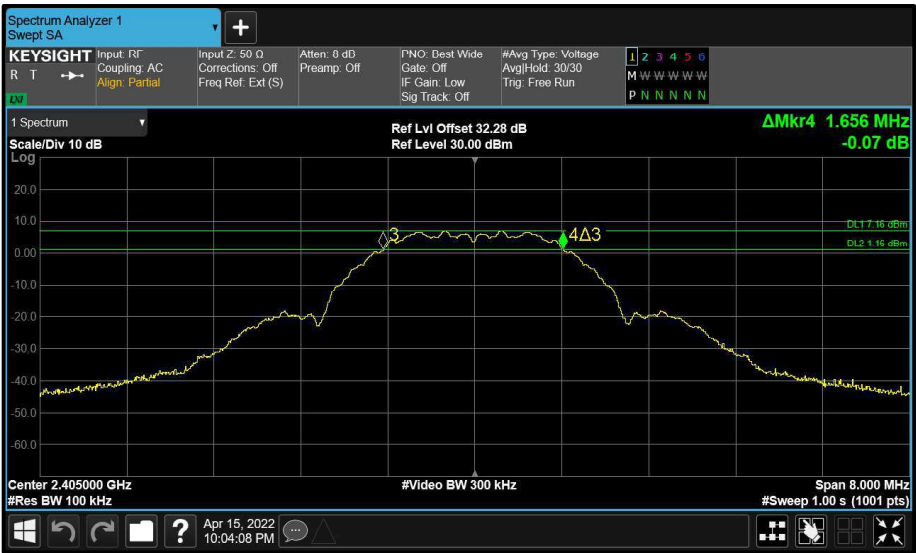
Figure 8 - A (A) 2405 MHz (CH11) 6 dB Bandwidth
