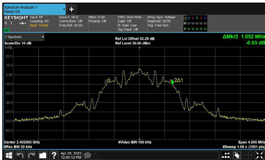
Figure 19 - Main (A) 2402 MHz (CH37) 99% Bandwidth
