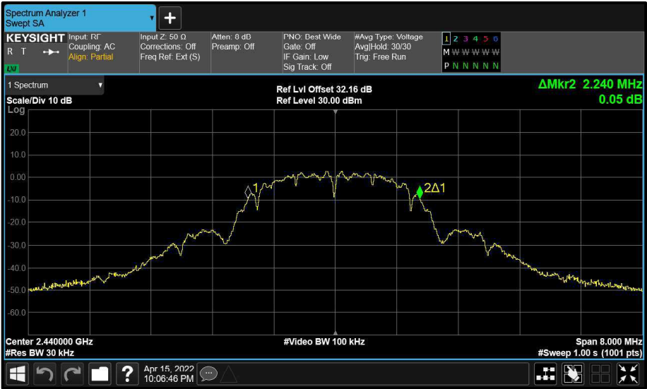
Figure 9 - A (A) 2440 MHz (CH18) 99% Bandwidth
