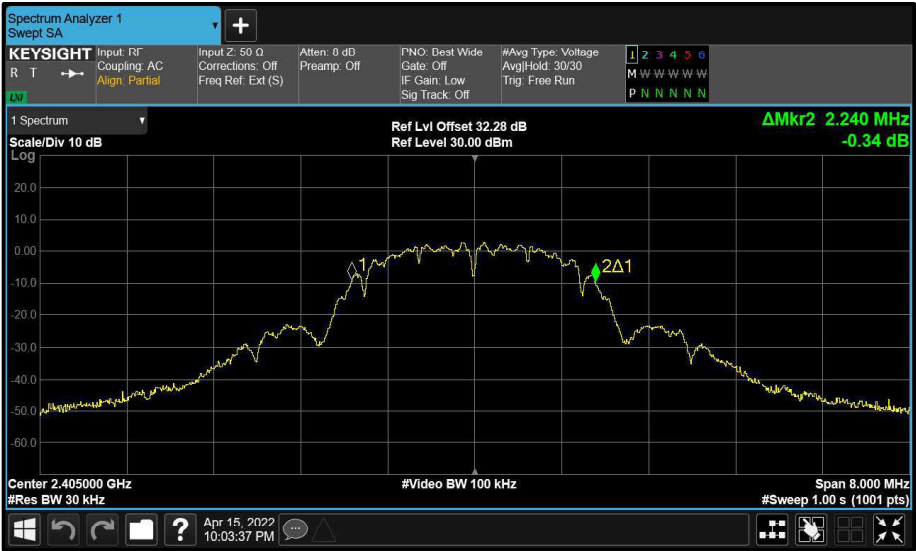
Figure 7 - A (A) 2405 MHz (CH11) 99% Bandwidth
