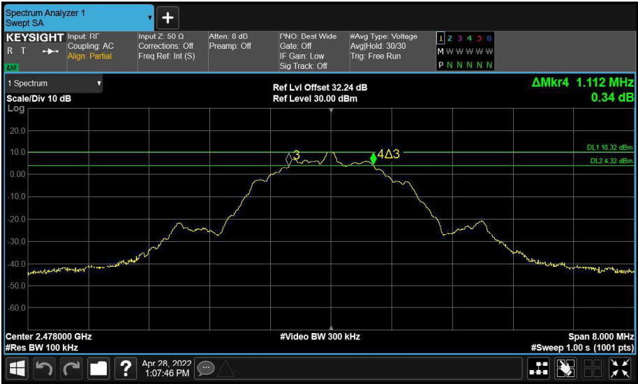
Figure 18 - Main (A) 2478 MHz (CH36) 6 dB Bandwidth
