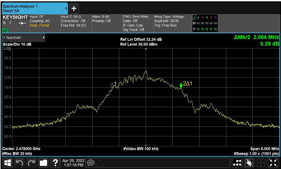
Figure 17 - Main (A) 2478 MHz (CH36) 99% Bandwidth
