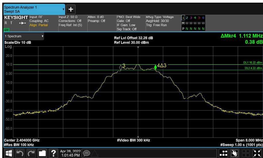
Figure 14 - Main (A) 2404 MHz (CH0) 6 dB Bandwidth
