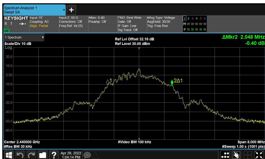
Figure 15 - Main (A) 2440 MHz (CH17) 99% Bandwidth
