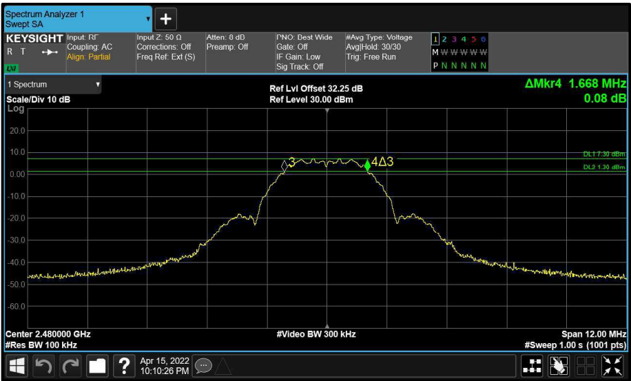
Figure 12 - A (A) 2480 MHz (CH26) 6 dB Bandwidth
