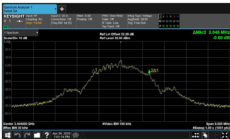
Figure 13 - Main (A) 2404 MHz (CH0) 99% Bandwidth
