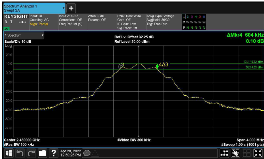
Figure 24 - Main (A) 2480 MHz (CH39) 6 dB Bandwidth
