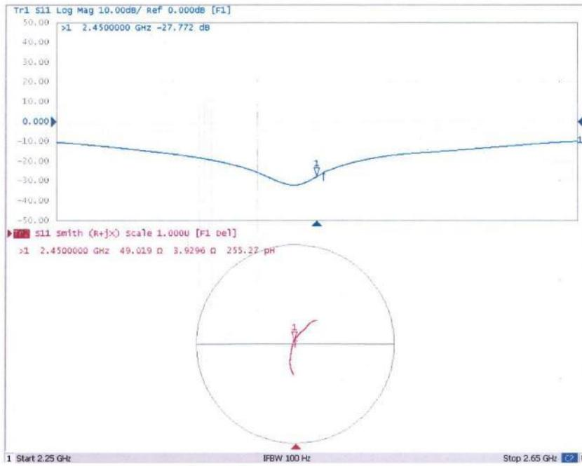
D2450V2 Dipole impedance and return loss Validation
