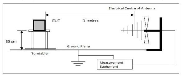
Above 1GHz, the EUT is raised using a low permittivity material (polystyrene) to a height of 1.5m.
