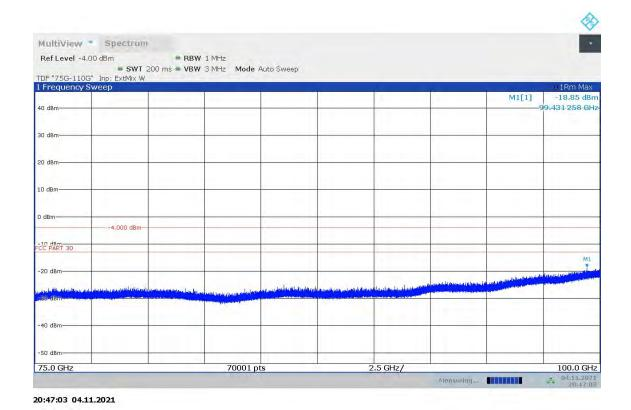
n261, Module0, 100MHz, PUSCH DFT, QPSK, 100%RB, Mid channel, 75GHz-100GHz, V
