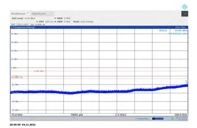
n261, Module0, 100MHz, PUSCH DFT, QPSK, 100%RB, Low channel, 75GHz-100GHz, H
