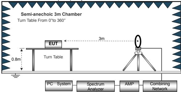
(B) Radiated Emission Test-Up Frequency 30MHz~1GHz
