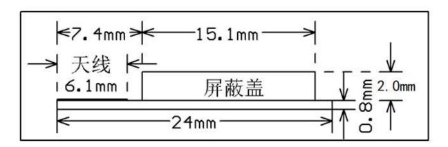
Note: The default dimensional tolerance is  $\pm 0.35$  mm. If you have specific requirements on dimensions, make them clear in the datasheet after communication.
