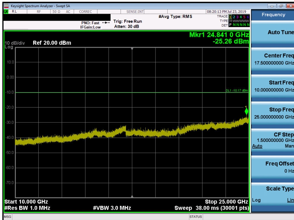
Plot 7-37. Conducted Spurious Plot (Bluetooth, 3Mbps – Ch. 0)
