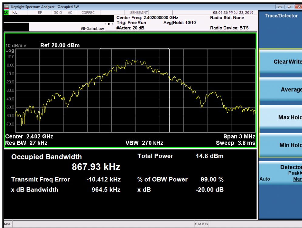
Plot 7-1. 20dB Bandwidth Plot (Bluetooth, 1Mbps – Ch. 0)
