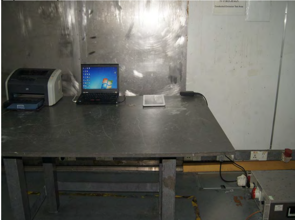
Photograph 2: Set-up for Spurious Emissions below 30MHz
