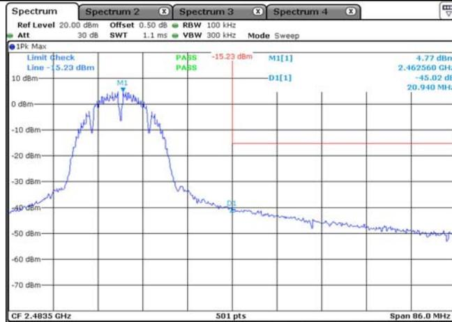
100 kHz Bandwidth of Frequency Band Edge
