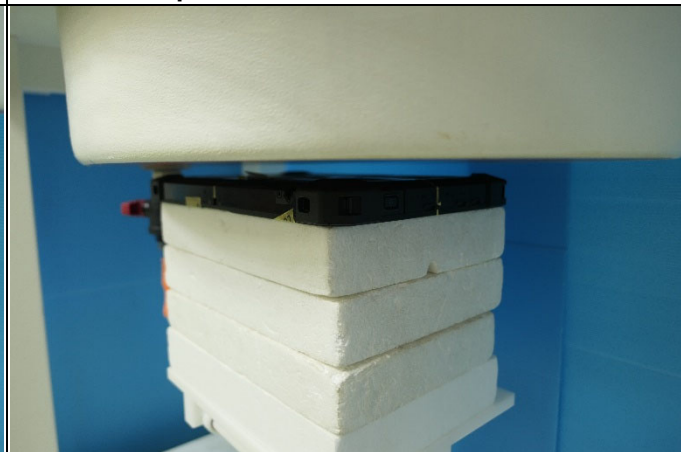
Back Side of EUT Tested at 11 mm
