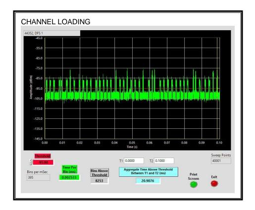
The level of traffic loading on the channel by the EUT is 20.9076%.
