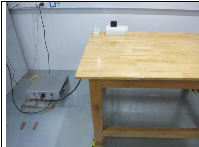
Conducted Emissions Test Setup Front View
