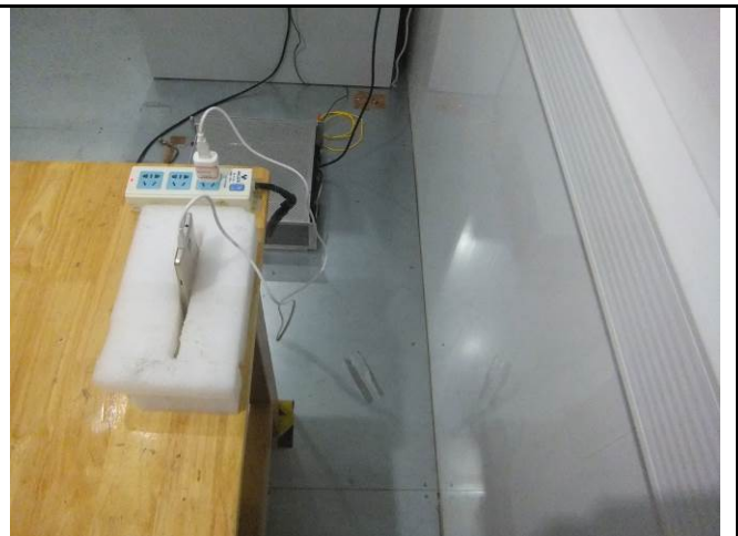
Conducted Emissions Test Setup Side View
