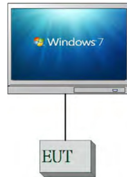
Fig 2-3 Conducted (AC Power Line) Configuration
