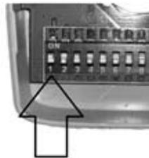
3. Using a paper clip or pen match the code to your receiver which was determined in step 1. The switch has an on and off position which is selected by gently pressing up or down.
