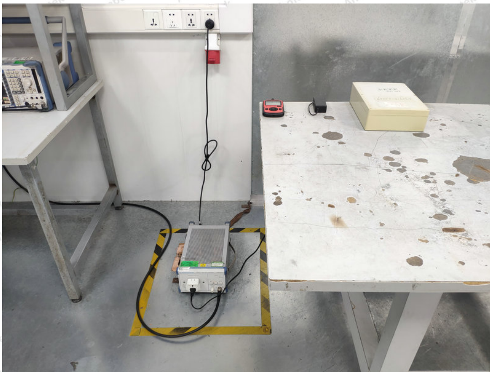
Photo of Power Line Conducted Emission Test
