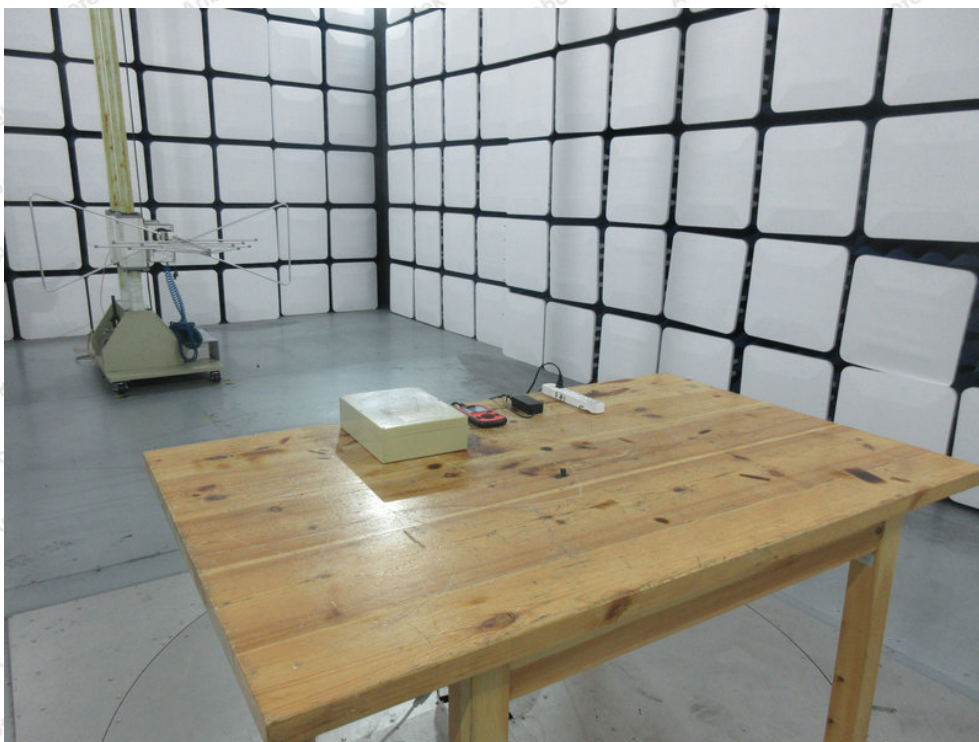
Photo of Radiation Emission Test
