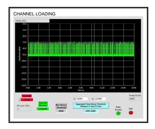
The level of traffic loading on the channel by the EUT is 19.872%
