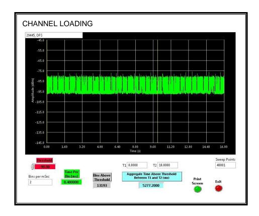
The level of traffic loading on the channel by the EUT is 52.77%
