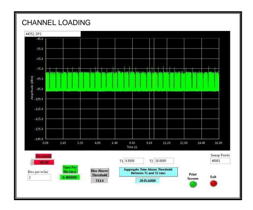
The level of traffic loading on the channel by the EUT is 28.456%
