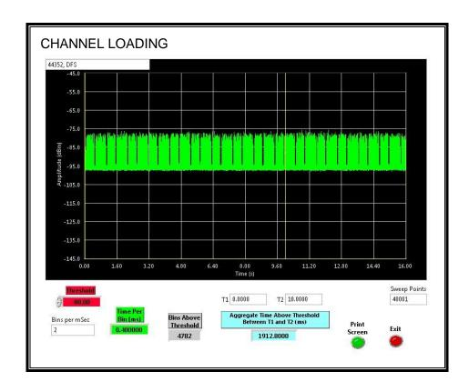
The level of traffic loading on the channel by the Peer Slave is 19.128%
