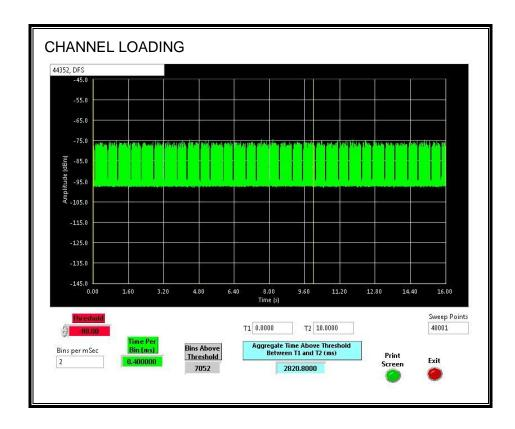
The level of traffic loading on the channel by the Peer Slave is 28.208%
