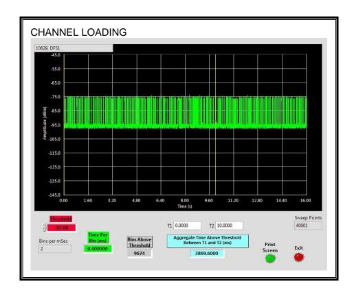
The level of traffic loading on the channel by the EUT is 38.696%
