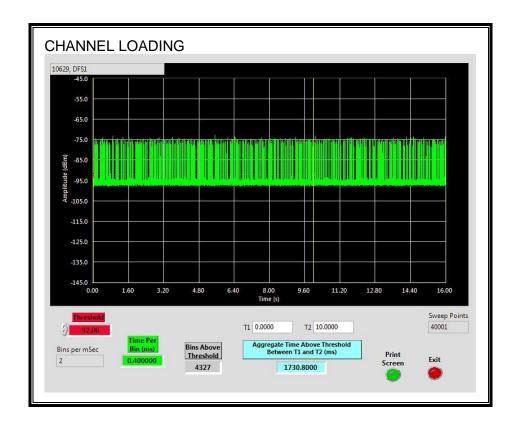
The level of traffic loading on the channel by the EUT is 17.308%
