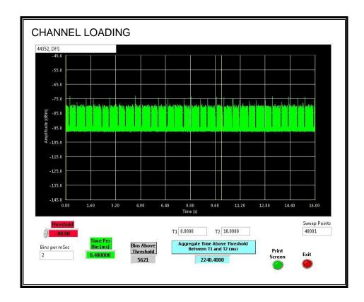
The level of traffic loading on the channel by the EUT is 22.484%
