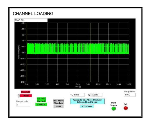
The level of traffic loading on the channel by the EUT is 17.53%
