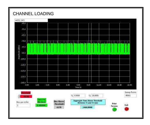
The level of traffic loading on the channel by the EUT is 24.68%
