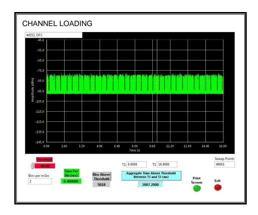
The level of traffic loading on the channel by the Peer Slave is 20.072%
