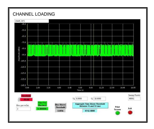
The level of traffic loading on the channel by the EUT is 47.42%
