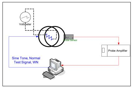
Figure 4-1 Validation Setup with Helmholtz Coil
