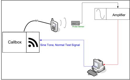
Figure 4-2 T-Coil Test Setup
