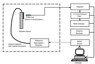
Figure 4-12 **Audio Magnetic Field Test Setup**
