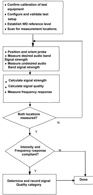
Figure 4-13 C63.19 T-Coil Signal Test Process
