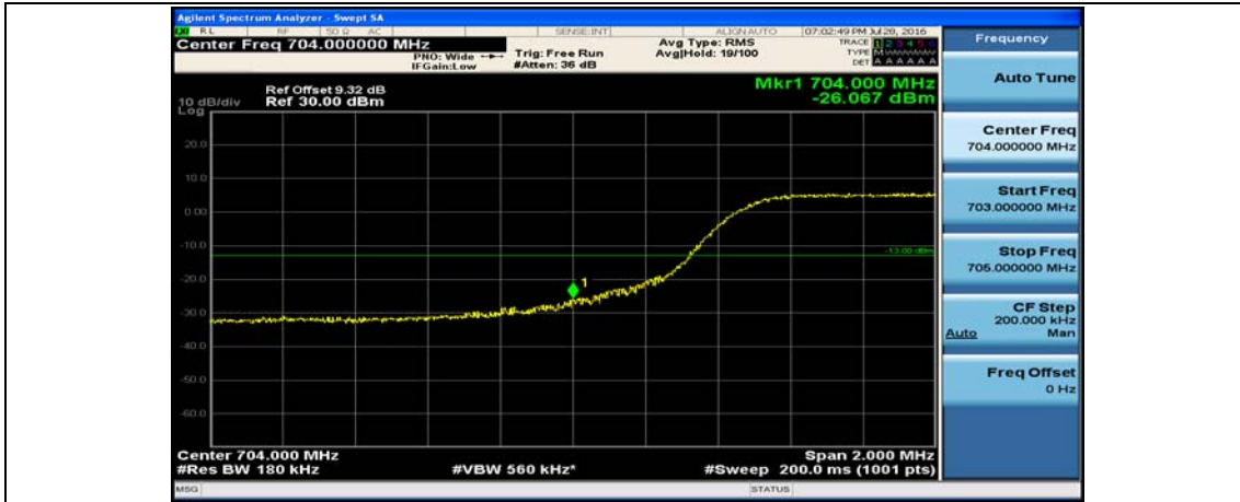
Channel Bandwidth: 10 MHz_HCH_16QAM_1RB#0
