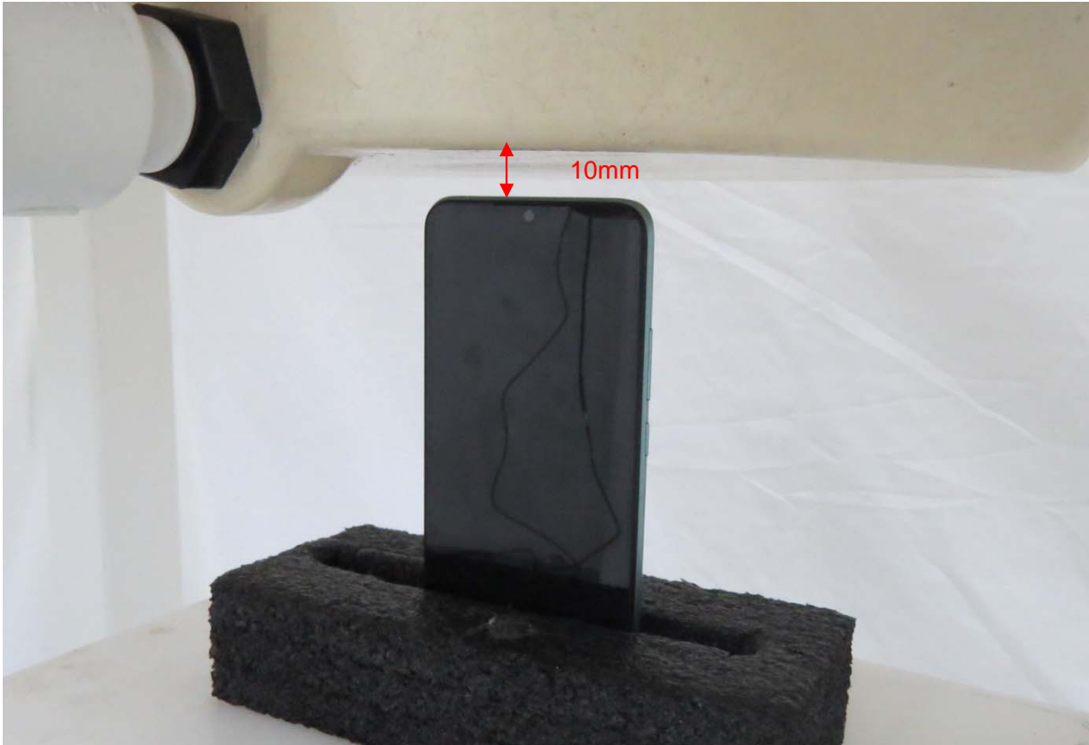
Picture 9: Top Edge, the distance from handset to the bottom of the Phantom is 10mm
