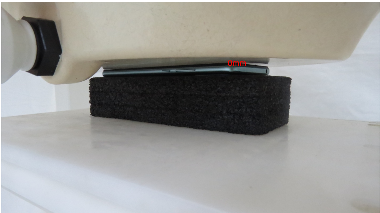
Picture 12: Front Side, the distance from handset to the bottom of the Phantom is 0mm
