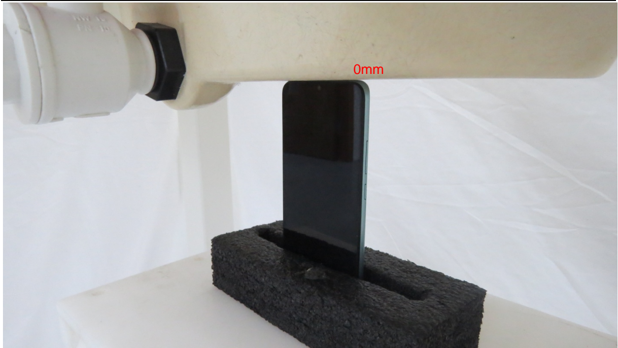
Picture 13: Top Edge, the distance from handset to the bottom of the Phantom is 0mm
