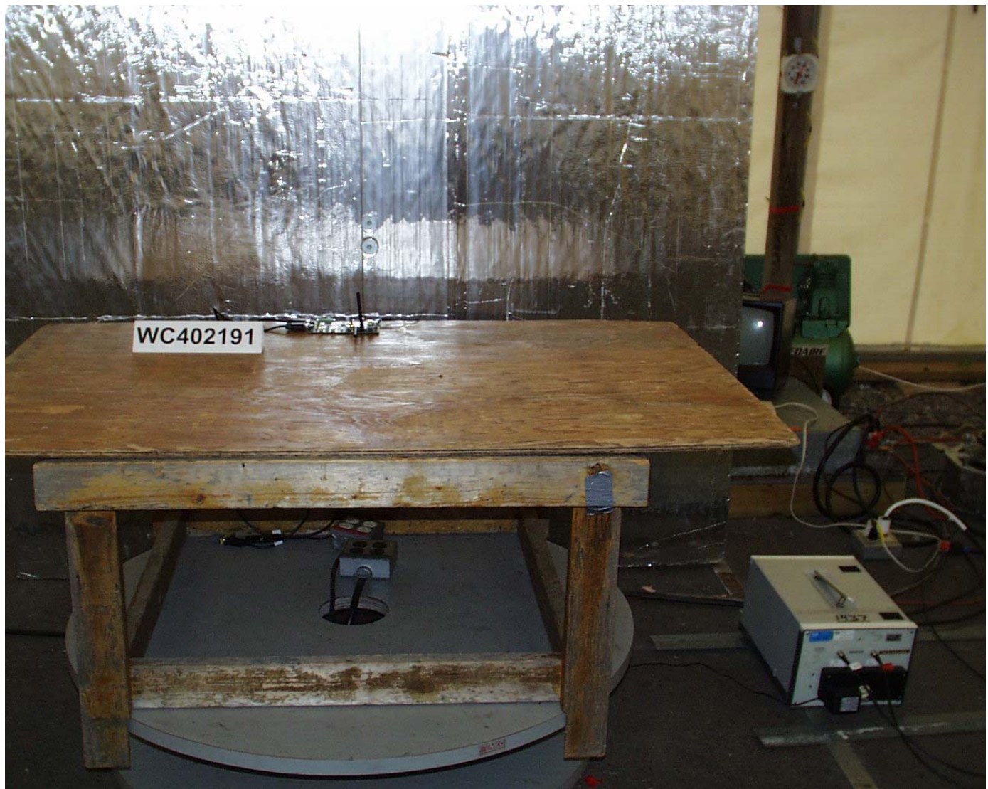
Test-setup photo(s): Conducted emission 150 kHz - 30 MHz
