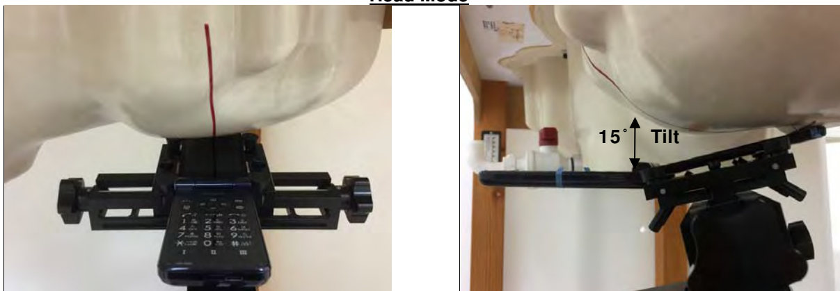
Fig.6 Left Head Section / Ear-Tilt Position(15°)
