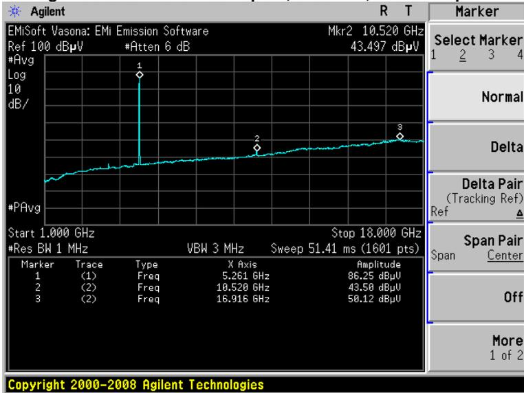
**Average Radiated Transmitter Spurs, 5300 MHz, 6 to 54 Mbps**
