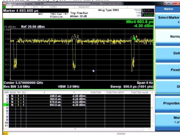
The Duty cycle of 160MHz BW is 95%, a 0.2dB CF is added to measurements.
