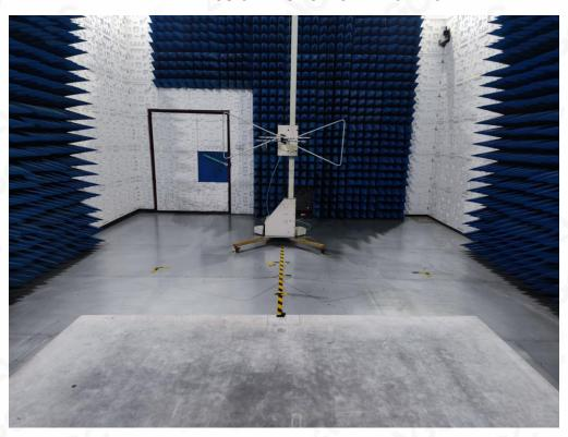
RADIATED EMISSION TEST SETUP ABOVE 1GHz
