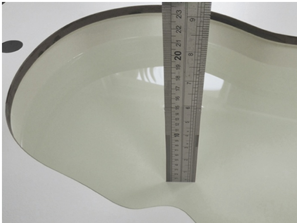
Liquid depth in the head phantom (2450MHz)
