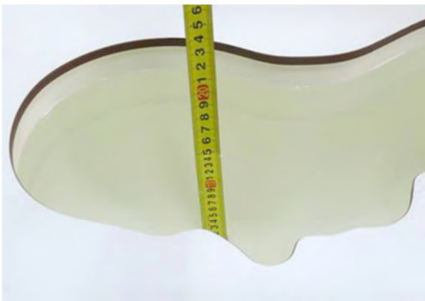
Liquid depth in the head phantom (835MHz)
