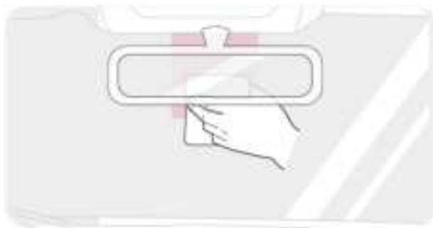
8. Peel off the protective sheet of 3M adhesive tape and attach the bracket base at the position of windshield vertically.
