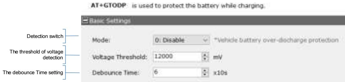
\*For the private car, taxi that using 12V vehicle battery, the threshold value should be less than 12000mV. 10000mV and 115000mV are recommended.
