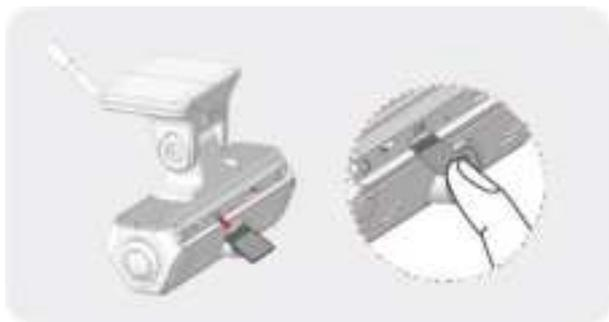
\*Before inserting the TF card, ensure that the metal contacts on the TF card are facing towards the mount connector of the product.
