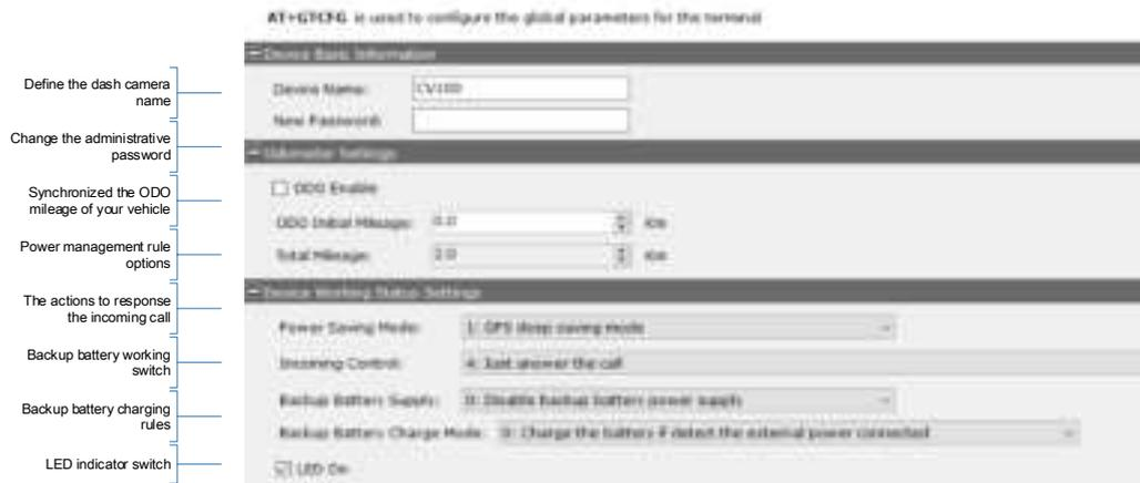
\*You must enable the “Backup Battery supply”, otherwise parts of features may be invalid.
