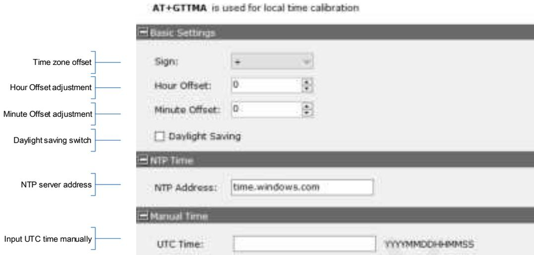
\*The priority of calibrating the system time: Manual Time < NTP Time < GPS Time.
