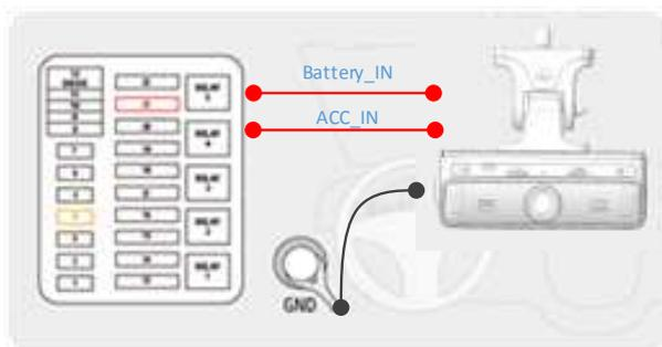
3. Close the vehicle fuse box and turn on ACC to check that the product is powered on.
