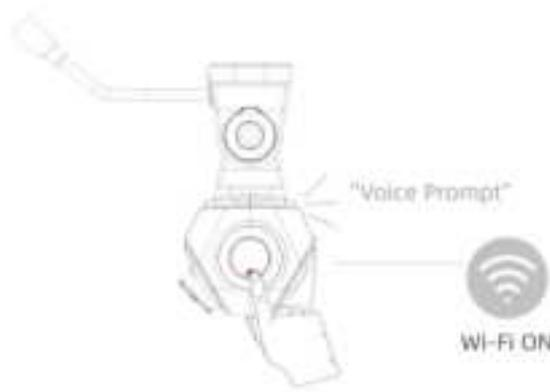
\*The WiFi of product automatically enables the “AP mode” and keep waiting for connections.it will be closed if no connected client after 5 minutes.
