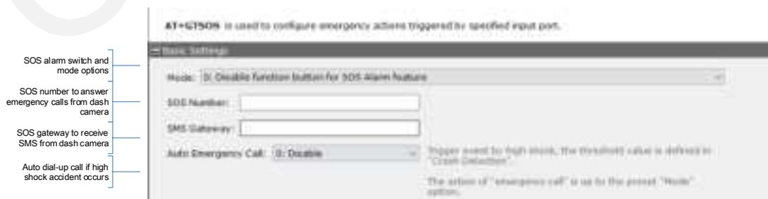
\*The responds depend on the Mode setting, the product can make the SOS call to the preset number, send the SOS alarm notification to the report server, or send the SMS message to the preset SMS gateway attached the location by google map link.
