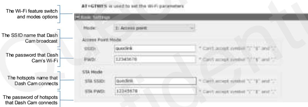
\* The product supports 2.4Ghz WiFi radio, please configure it to connect the 2.4Ghz access point while it's working in STA mode.
