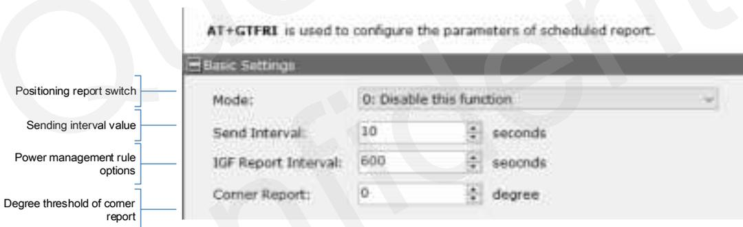
\*Enable the FRI feature to receive the coordinate information and track the vehicle at any time.
