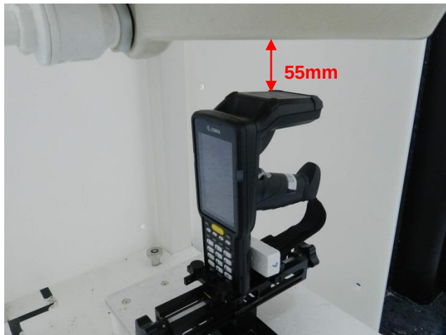
Front, Test Separation 55 mm
