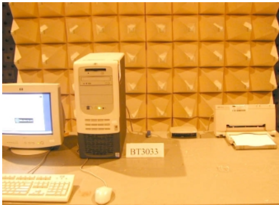
Photo 1: Spurious Test Set-up photo (front)
