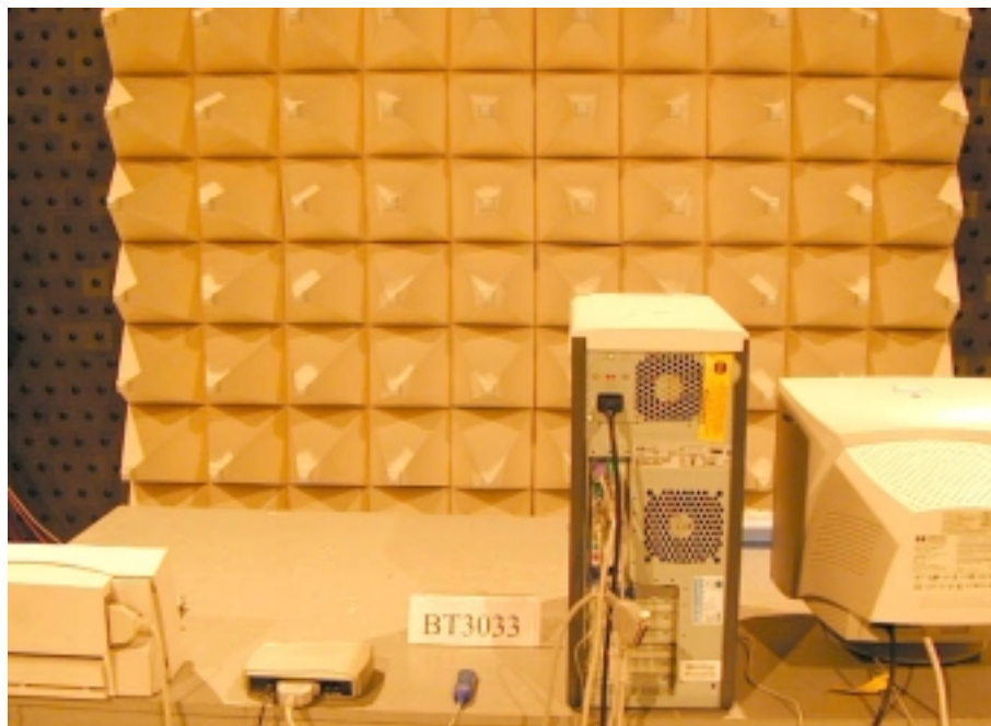
Photo 2: Spurious Test Set-up photo (rear)
