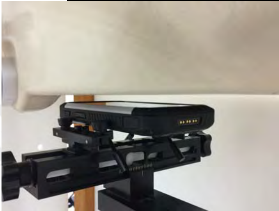
Fig.9 EUT Front side to flat phantom
