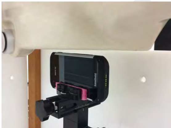
Fig.14 EUT Right side to flat phantom
