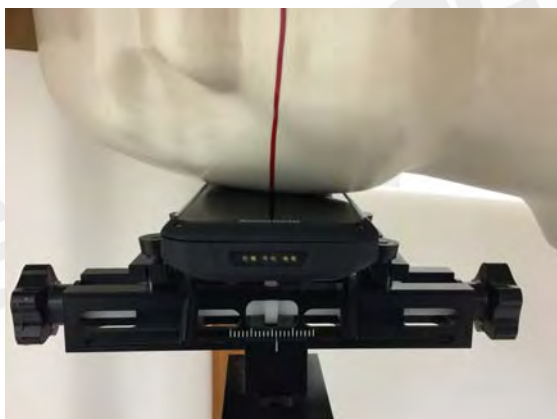
Fig.3 Right Head Section / Cheek-Touch Position
