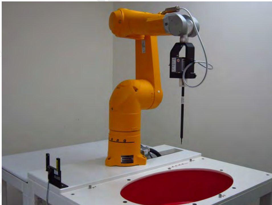
Fig.1 Photograph of the SAR measurement system
