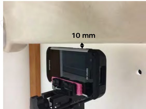
Fig.13 EUT Left side to flat phantom
