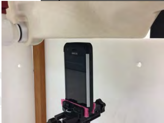
Fig.12 EUT Top side to flat phantom
