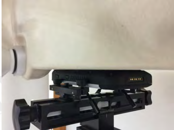
Fig.15 EUT Back side to flat phantom
