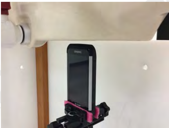
Fig.10 EUT Bottom side to flat phantom
