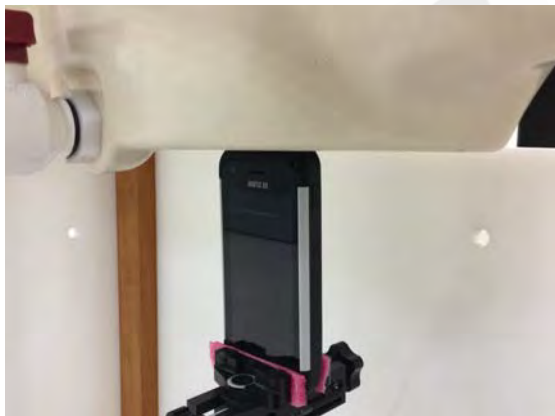
Fig.17 EUT Top side to flat phantom
