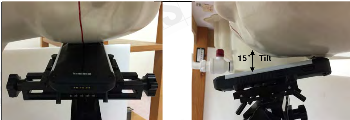
Fig.6 Left Head Section / Ear-Tilt Position(15°)
