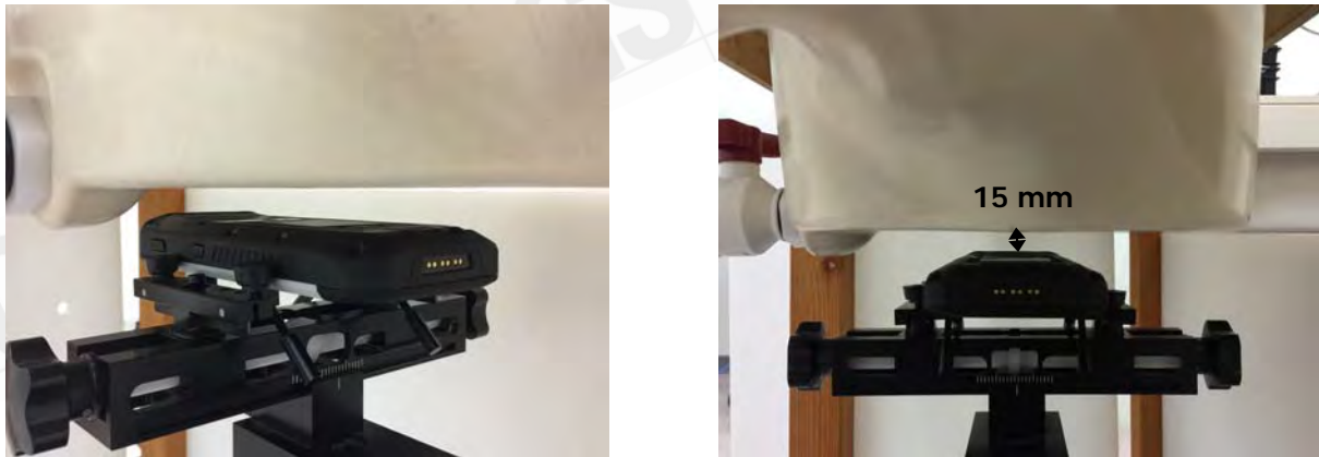
Fig.8 EUT Back side to flat phantom
