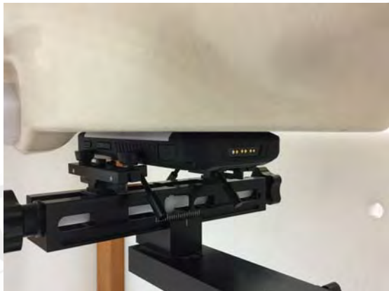
Fig.16 EUT Front side to flat phantom
