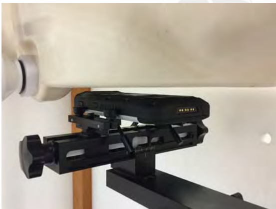
Fig.11 EUT Back side to flat phantom
