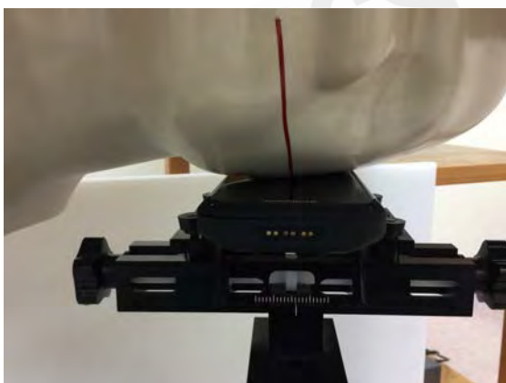
Fig.5 Left Head Section / Cheek-Touch Position
