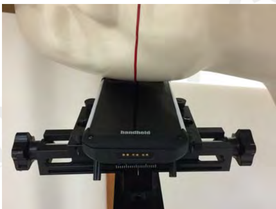
Fig.4 Right Head Section / Ear-Tilt Position(15°)
