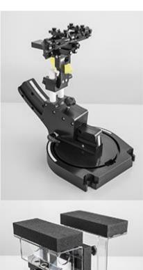
The DASY device holder is designed to cope with the different positions given in the standard. It has two scales for device rotation (with respect to the body axis) and device inclination (with respect to the line between the ear reference points). The rotation center for both scales is the ear reference point (ERP). Thus the device needs no repositioning when changing the angles.
