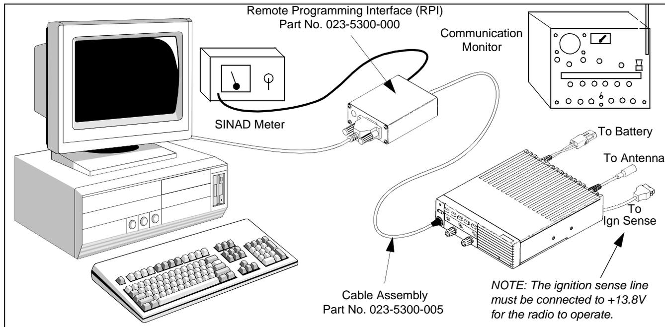
Figure 6-1 Alignment Setup
