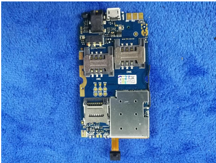
Mainboard with Shielding - Front View
