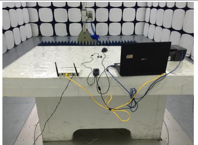
Radiated Emissions Test Setup Above 1GHz
