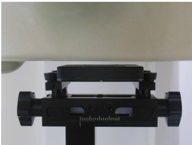
Back, Test Separation 0.5 cm
