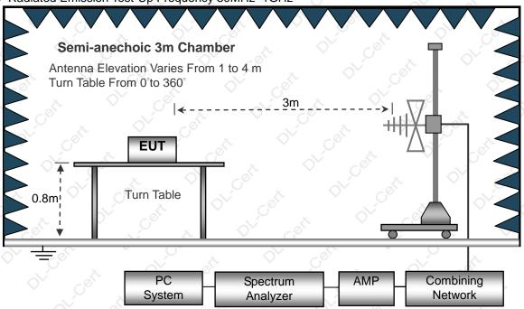
(C) Radiated Emission Test-Up Frequency Above 1GHz
