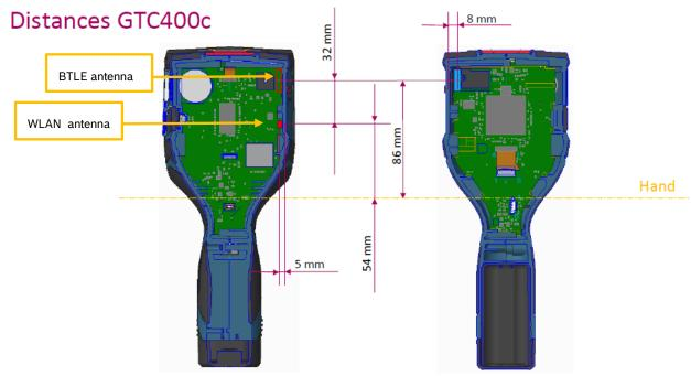
The dimensions of the product GTC400C, shown above, are: 233mm x 95mm x 63 mm (length x width x height)
