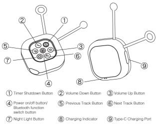
1.Charging: Charging indicator turns red during charging and green when fully charged. Charging Time: 2.5 hours (0% to 100%).
